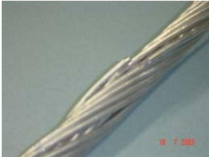
Figure 1. A broken strand on an AAAC conductor three years after construction.
